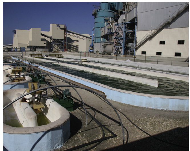
Fig. 1. Algae ponds at Seambiotic, Inc. in Ashkelon, Israel. Parts of a 4 GW fossil fuel burning power plant are in the background.
